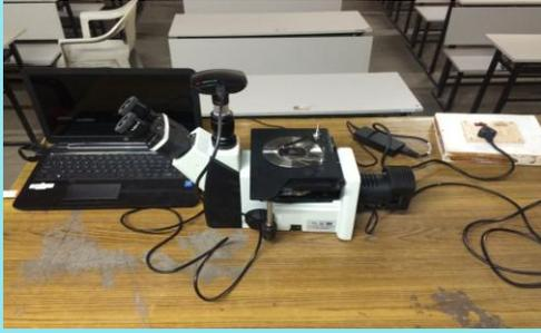
**Motorized Stage Metallurgical Microscope**
